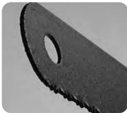
The **thickness** of a hacksaw blade is about **1 mm**.
